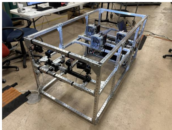
Fig 2. Electrochemical Cells Mounted in the Flight Payload
